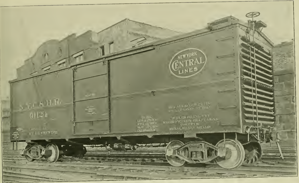
Steel End Applied to Experimental Steel Box Car; New York Central & Hudson River.
